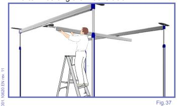
31) Centre the mobile track to make it protrude equally on each side.
