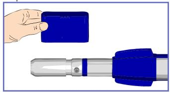
Slide the locking handle upward and remove the blue plastic strips from each side of the posts. Gently pull out the end.
