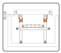
Check to ensure that the height of the bottom of the bath base track  $\stackrel{\frown}{(\mathbb{A})}$  is higher than the bath threshold  $\stackrel{\frown}{(\mathbb{B})}.$
