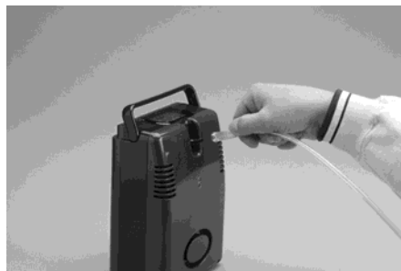
Figure 9: Connecting Cannula to FreeStyle's Oxygen Outlet
