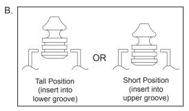
Insert pillows as shown into the corresponding grooves on the cushion to achieve the desired pillow height position.
