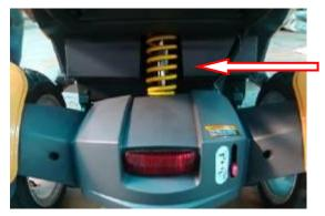
The softness of the rear suspension system is adjustable. There are altogether 5-level of adjustments. It is applicable with around 120kg and each level can bear up to 13.5 kg.
